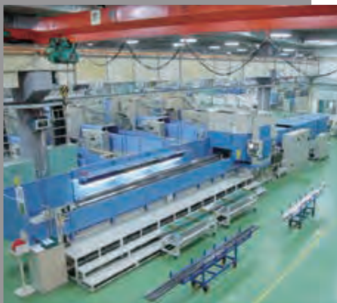
7-meter grinding machine for LM rails LM轨道7m磨床
