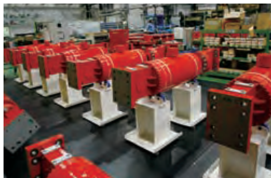
Viscous Damping System RDT 减振装置RDT
